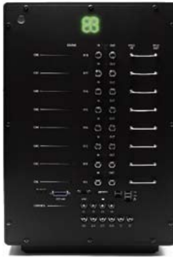
The EB Propsim radio channel emulator replaces the real-world radio channel between transmitter and receiver to bring air-interface testing into the lab. Aircell employed the instrument to help develop and test its Gogo Internet service for commercial airplanes. Courtesy of Elektrotbit.
